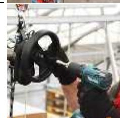
Note: Always use the slowest gear of the battery screwdriver (max. 350 rpm); suggested minimum torque 20N.m
